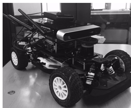
Fig. 1-1. An MIT RACECAR as used in summer 2016. This vehicle does not use the structure.io depth camera and has a router mounted directly to the top of the chassis.
