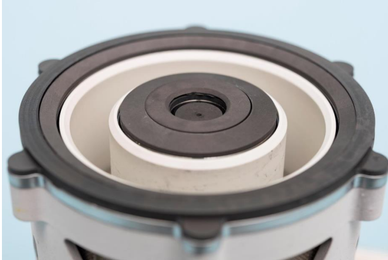
Figure 4. The graphite pole covers on the MaSMi-EM SN001 Hall thruster.
