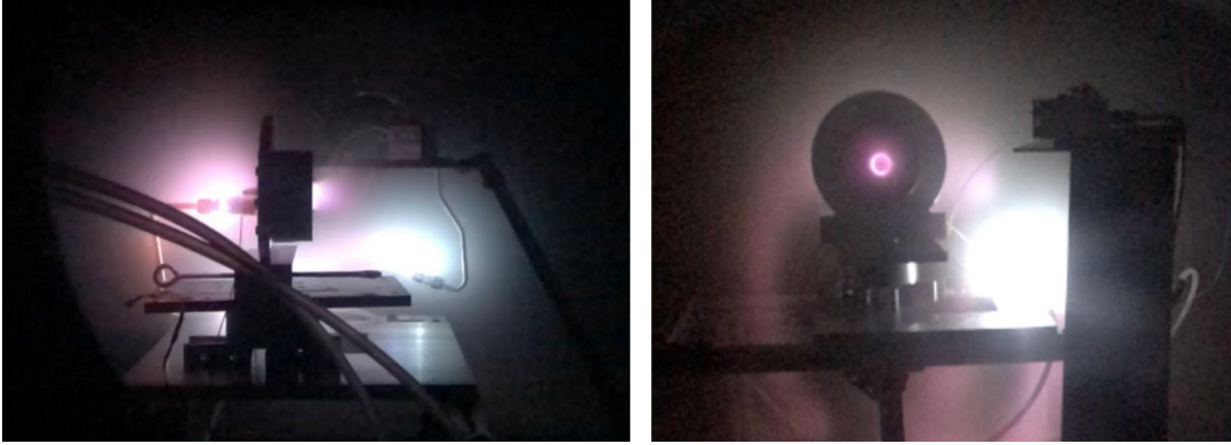
FIG. 14. Thrust pulses captured from the side (left) and front (right) of the thruster. The pink glow is characteristic of an Argon plasma.
