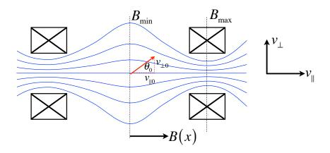
Through a more detailed analysis of magnetized particle motion, it is found that in addition to the conservation of energy (kinetic only in this case, if there is no electric potential),
