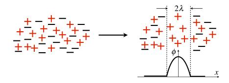
The plasma is quasineutral everywhere  $(n_e \approx n_i)$  except in the region where a net positive charge exists. In general, Poisson's equation Eq. (6) describes the electric potential for a given charge distribution,
