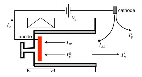
Where  $V_a$  is the accelerating voltage and  $I_a$  the current through the power supply (or anode current, or also cathode current). Of the  $I_a$  current of electrons injected by the cathode, a part  $I_B$  goes to neutralize the beam, and the rest,  $I_{BS}$  back-streams into the thruster. Since no net current is lost to the walls,
