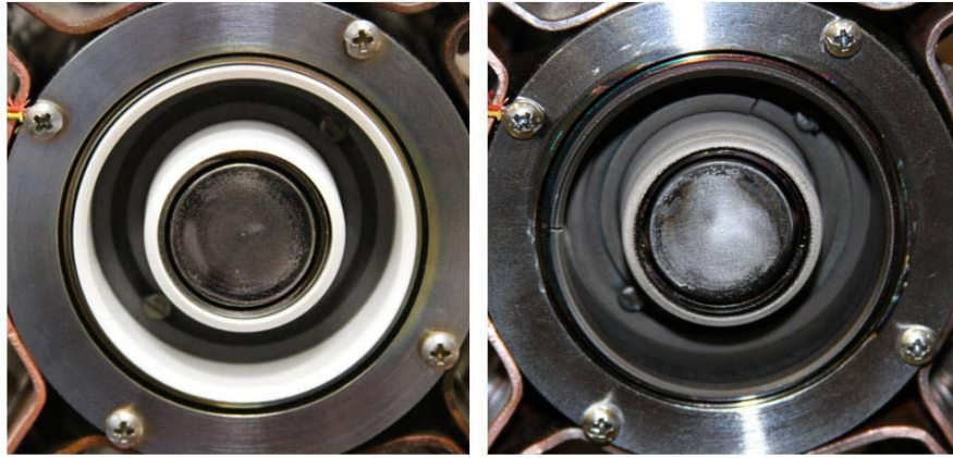
Fig. 11. Comparison of MaSMi's discharge channel before (left) and after (right) testing. The layer of carbon back-sputter suggests the presence of magnetic shielding.
