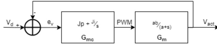
Figure 2: Block diagram of the motor/motor-controller subsystem showing frequency response equations in the s-domain.
