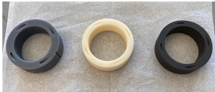
Fig. 7 Photograph of three diffuser prototypes. Left: low-temperature SLA resin used to prototype the dimensions for the ceramic diffuser. Center: high-temperature SLA resin prototype (Somos PerFORM) used in the tested thruster configuration. Right: aluminum DMLS prototype with black anodized coating to ensure electrical insulation
